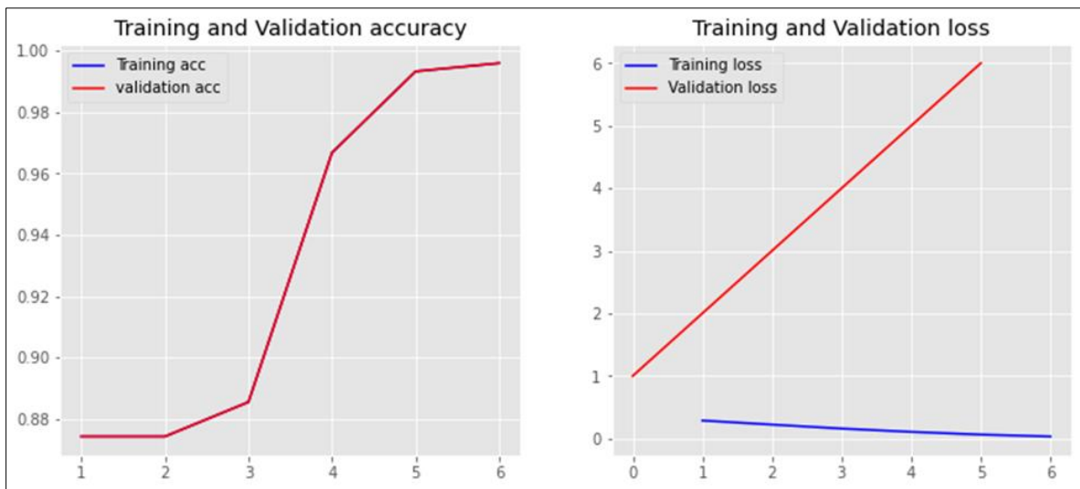
Figure 12 Training and validation accuracy and loss graphs
