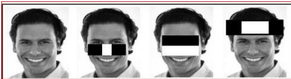
Figure 3 Examples of Haar features. Areas of white and black regions are multiplied by their respective weights and values added [29]
